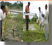
Carry out the field re-survey Referring to Form A data using DGPS/ETS
