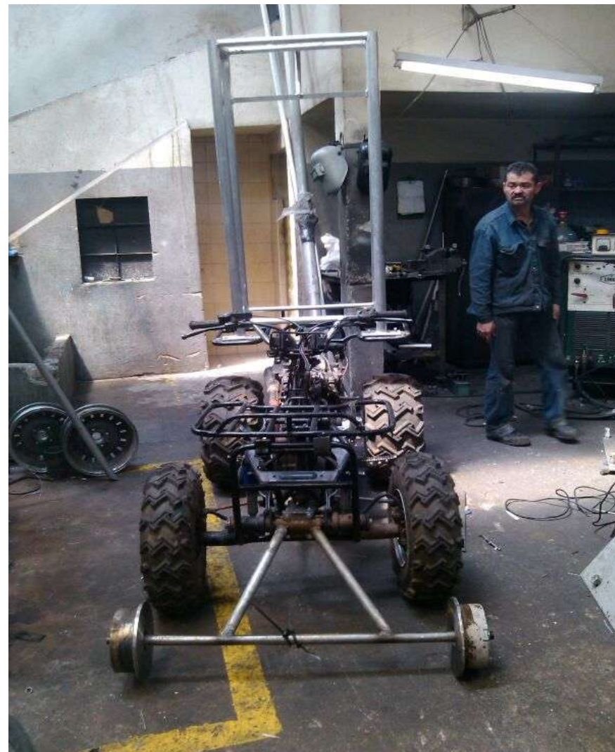
Fabricating mobile LiDAR mount and rail ATV
