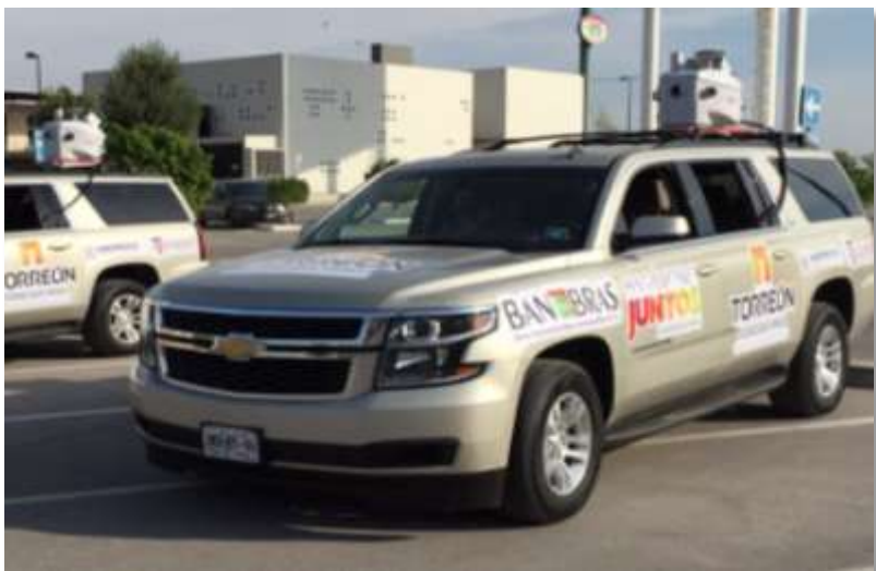
Leica Pegasus mobile LiDAR and 360 photography
