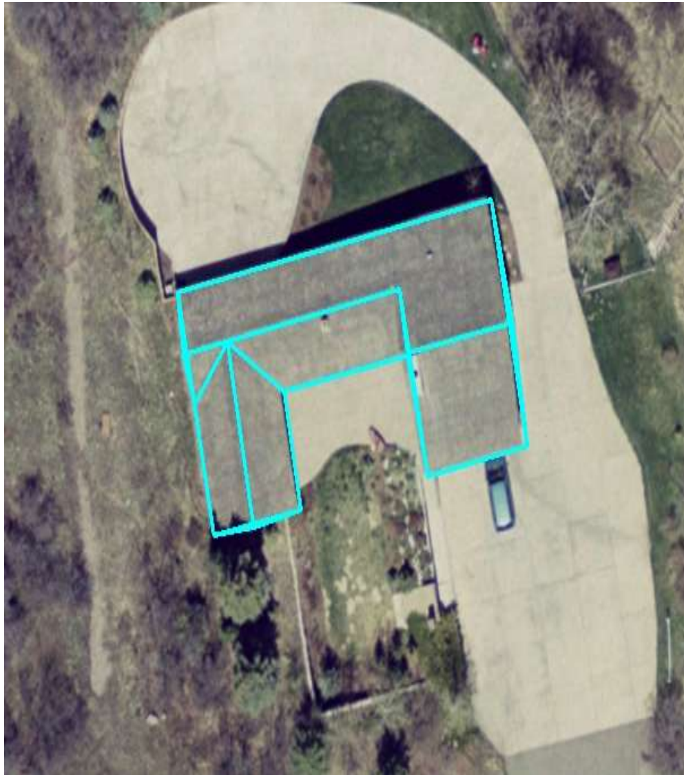
LiDAR creates building wire-frame and volumetry
