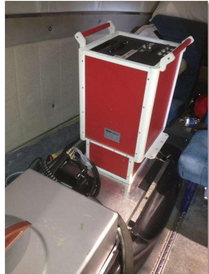
Co-mounted ITRES TABI-1800 Thermal Imager, Leica LiDAR, Trimble TAC camera
